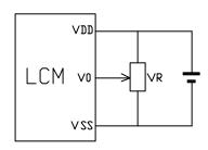
$V_{\text{DD-}}V_0\text{: LCD Driving voltage}$
